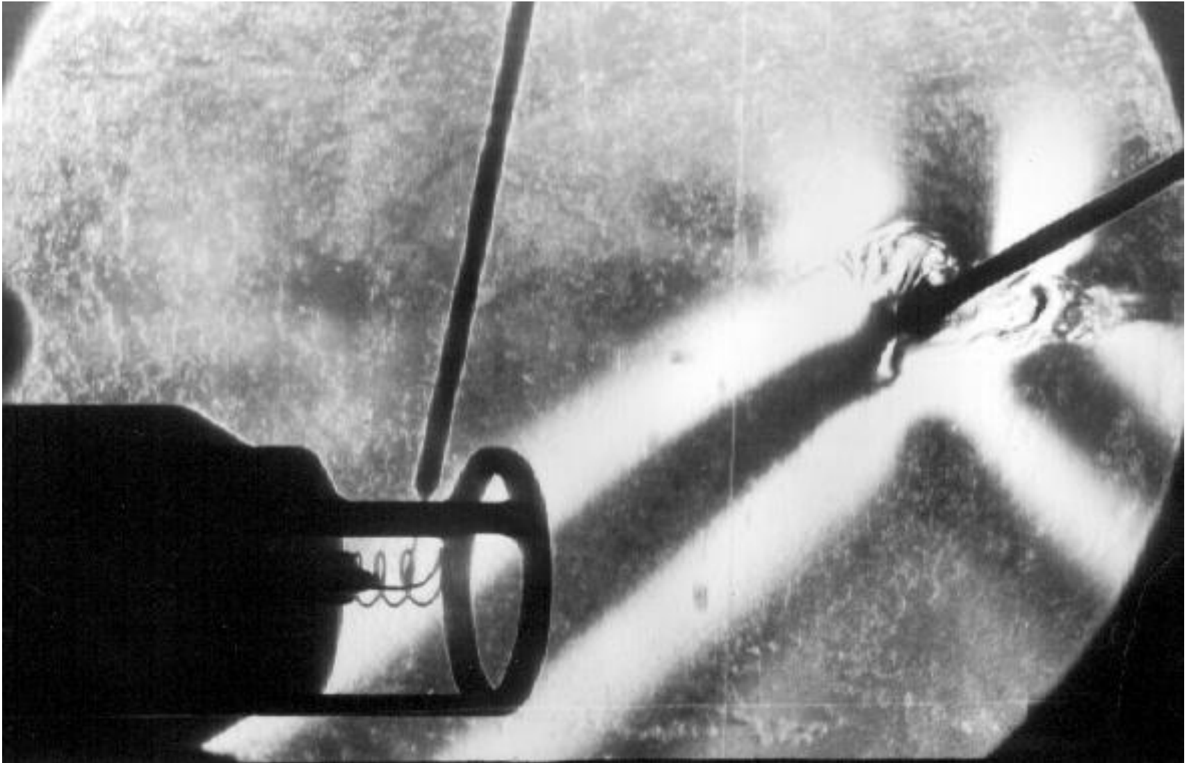
Pattern of periodic internal waves wedges contacting with conductivity probes in a fluid with variable buoyancy frequency
