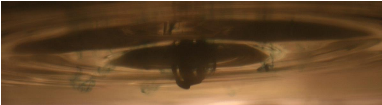
Flash and wakes of thin jets inside water layer produced by a drop of a ink solution
