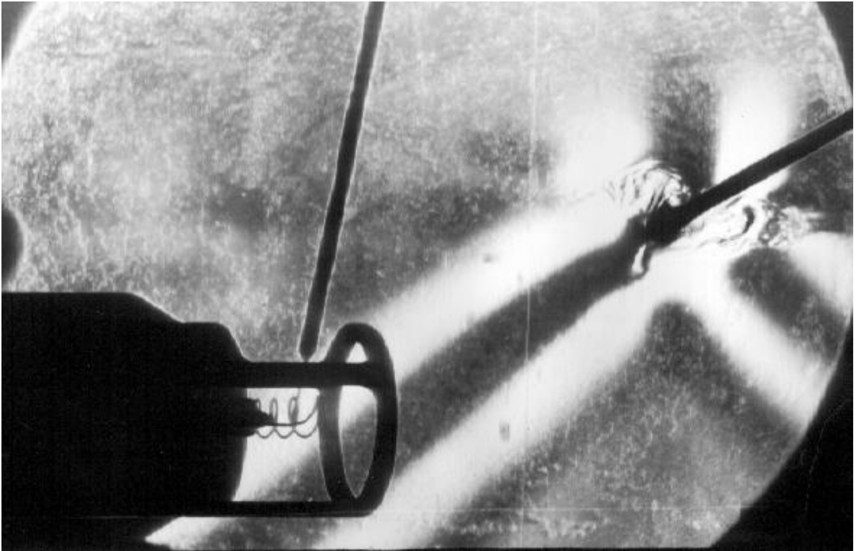
Pattern of periodic internal waves wedges contacting with conductivity probes in a fluid with variable buoyancy
