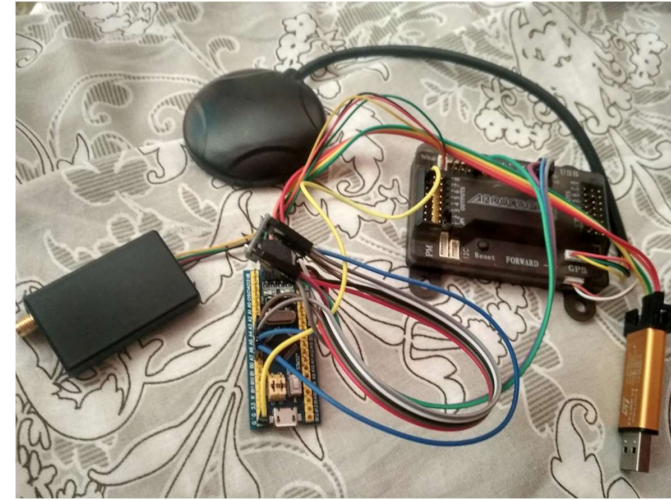
Fig. 16. Connection of the controllers using SPI bus
