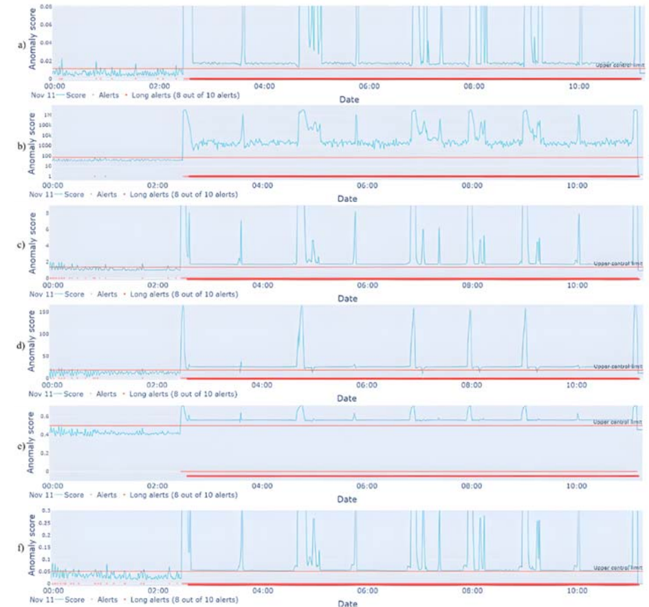
Fig. 12. Anomaly graphs for the test period of the HDFS dataset constructed by the following methods: a) Autoencoder, b) Elliptic Envelope, c) Local Outlier Factor, d) One Class SVM, e) Isolation Forest, f) k-Nearest Neighbours.
