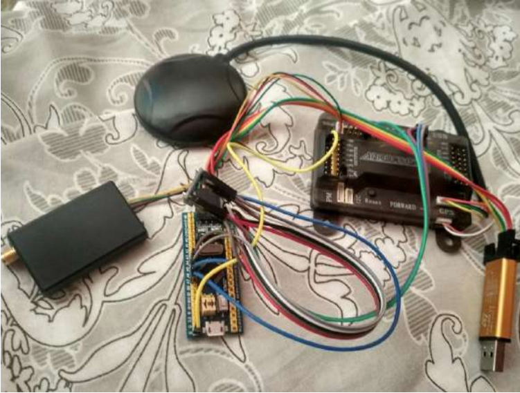
Fig. 16. Connection of the controllers using SPI bus
